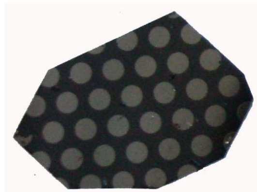
Fig. 1. Schottky contacts on the i-p+ SCCVD Diamond Sample.
