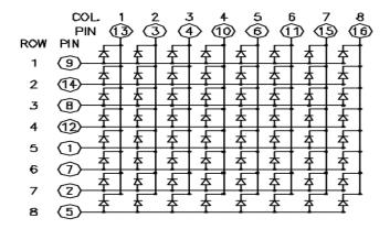
For one colour LED matrix there is no distinction between common cathode and common anode LED matrices. To make a particular LED glow make the row number pin High and the column pin Low. We can control all the LEDs in this way.
