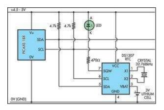
A real time clock is basically just like a watch - it runs on a battery and keeps time when there is a power outage. Using an RTC, you can keep track of long timelines, even if you reprogram your microcontroller or disconnect it from USB or a power plug.
