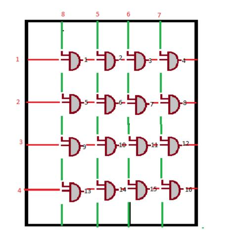
Here, we can see that the wires numbered from 1 to 8 represents the outputs coming from the Arduino board, and the wires numbered 1 to 16 are the outputs. We can see that if both the pins 1 and 8 are raised high, then the top most AND gate gives an output HIGH which is fed to the topmost LED. Thus the top most LED is represented as (1,5). So, the LEDs in the order are (1,8),(1,5),(1,6),(1,7),(2,8),(2,5),(2,6),(2,7),(3,8),(3,5),(3,6),(3,7),(4,8),(4,5),(4,6),(4,7).
