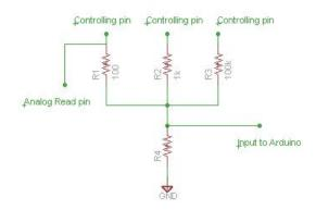
Figure 2: Voltage divider used to measure resistance
