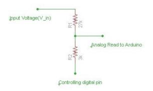
Figure 1: Voltage divider used for measuring voltage
