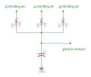
Figure 3: Voltage divider used to measure capacitance
