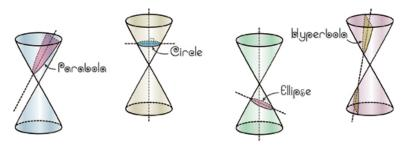
We will show that the curve r = r<sub>0</sub>/(1-εcosθ) in plane polar coordinates, denotes different conic sections for various values of ε, which is nothing but the eccentricity
