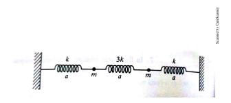
3. Two mass points of equal mass m are connected to each other and to fixed points by three equal springs of force constant k, as shown in the diagram. The equilibrium length of each sprint is a. Each mass point has charge +q, and they repel each other according to Coulomb law. Set up the secular equation for the eigenfrequencies.
